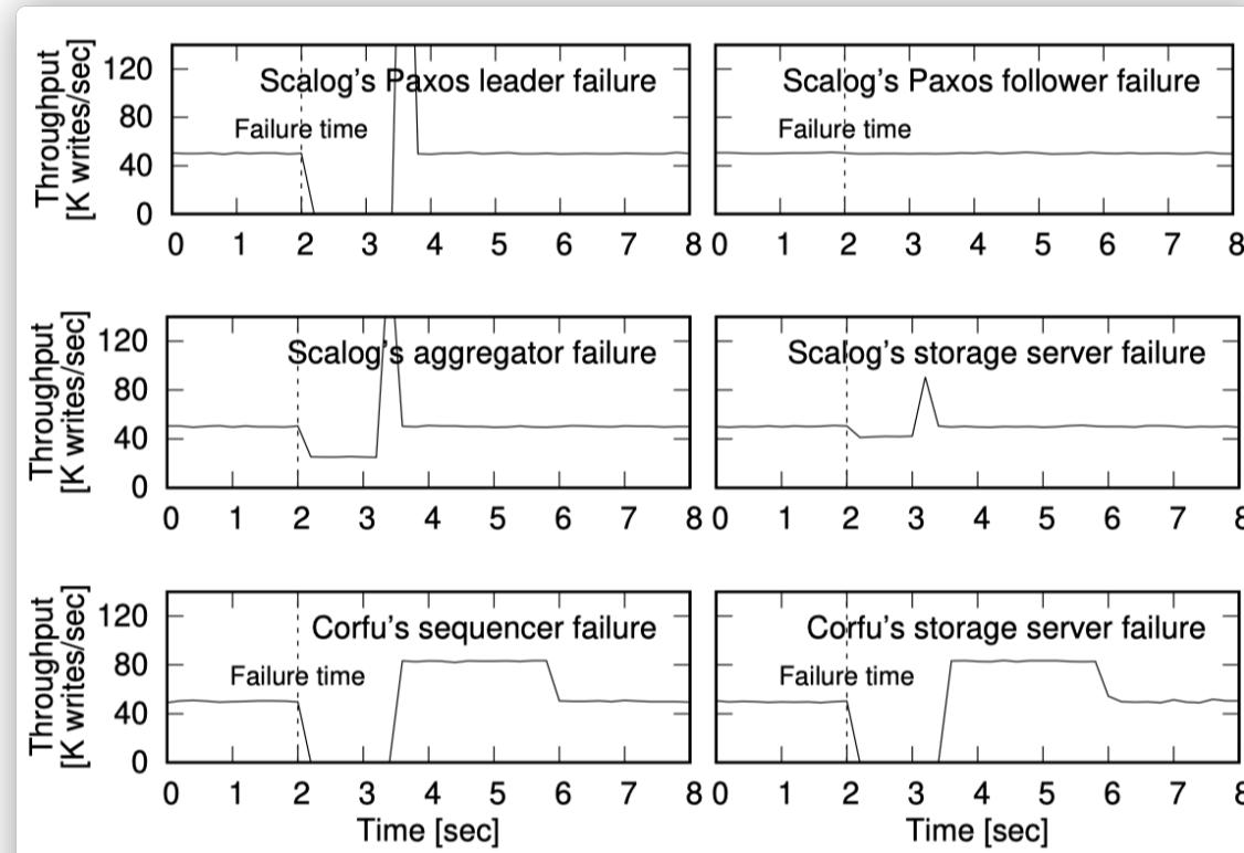
Figure 4: Throughput under different failure scenarios
